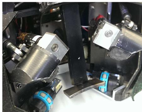
**Fig. 4.** Shooting lever end-effector for more accurate passing.
